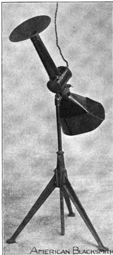
FIG. 1. ELECTRIC GAUGE FOR MEASURING HIGH TEMPERATURES.
