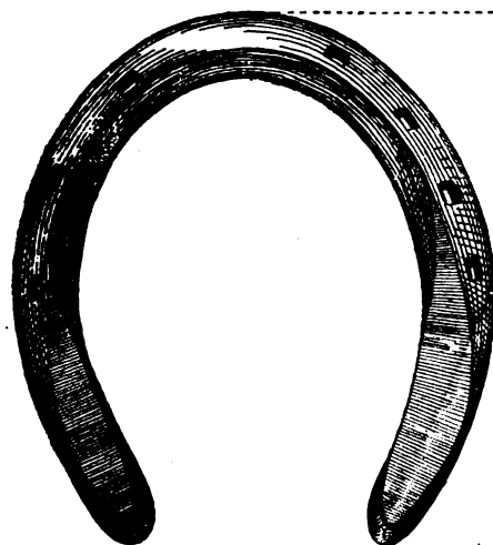
Fig. 18.—A HEEL-WEIGHT SHOE TO INDUCE HIGH ACTION.
