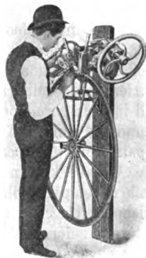
Fig. 5. BRAZING THE ENDS OF THE RETAINING WIRE TOGETHER.
