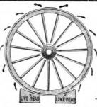
equally around the wheel at the same time, each head drawing one-half of tire.
