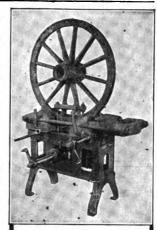
Hydraulic power has always been considered most valuable, and when applied to a side grip tire setter, it makes a machine that works easier and quicker than any other side grip machine in existence
