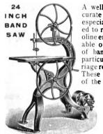
A well-made accurate machine; especially adapted to run by gasoline engine; capable of all kinds of band sawing, particularly carriage repair work. These are a tew of the fine points of Mars-ton's Band Saw.
