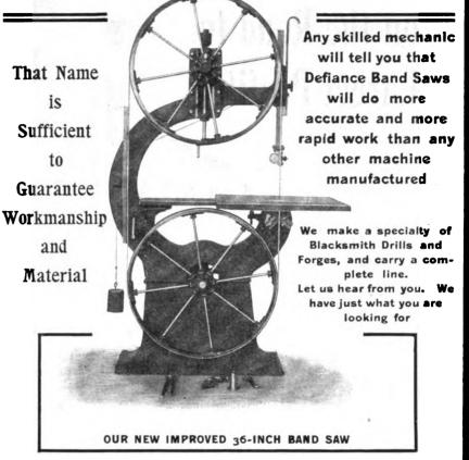
WHEELS-36 in. diameter, 2 in. wide. Made of either castiron or cold rolled shafting, with wooden rims covered with pure gum rubber, 1/2 in. thick. TABLE-Iron with wood center. Easily tilted and especially convenient for sawing bevel.
