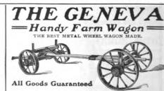
Pressed steel wheels, any height and width tire, interchange hubs. Gears of selected stock, thoroughy irone Made
