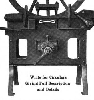
With this Machine the tire is first drawn tightly around the wheel, and then compressed within a space of ten inches instead of being bunched in one inch. The value of this principle can readily be seen
