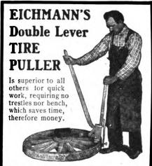
By using this tool it will save you the vexation of breaking up felloes and beating off tires. It is light and very easy to handle, yet powerful. 50 pounds on the lever lifts one ton on the hook. Though made especially for wide tires, yet you can use it as well to remove buggy tires.
