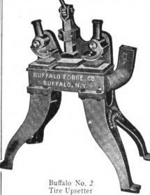
THIS machine upsets 3 x 5/8 tires and axles up to 1½ in. square. Grips are faced with tool steel with teeth carefully cut and tempered. Lower grips adjust themselves automatically to curvature of tire or for straight work. Upset both straight and curved work. The plunger prevents all buckling or kinking. Weight 275 lbs. Height 22 in. Write for circular.
