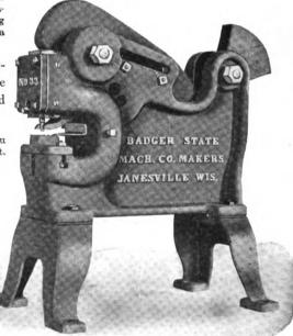
The body of this machine is cast in one piece (instead of being two pieces and bolted together) which we claim greatly strengthens the machine. All pins and king botts are made of steel. The madrel, which holds the punch, is made square to avoid turning and spoiling the dies when square or irregular shaped punches are being used, Angle shearing attachment can be furnished for this machine.
