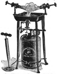
Patented February 7, 1900. The up-to-date machine for brazing agricultural implements, autômobiles, bicycles, etc. Will do all kinds of brazing, both light and heavy. It is fitted with three powerful improved Hydro Carbon Burners. Both Gasoline and Kerosene Machines in stock. Wite for description.
