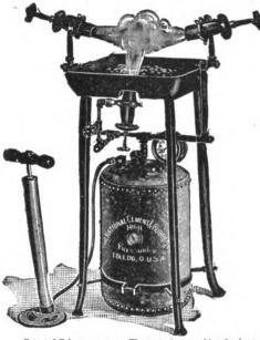
Patented February 7, 1900. The up-to-date machine for braz-ing agricultural implements, automobiles, bicycles, etc. Will de all kinds of brazing, both light and heavy. It is fitted with three powerful improved Hydro Carbon Burners. Both Gasoline and Kerosene Machines is voice. With for description
