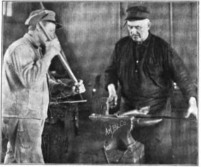
FIG. 5-BEND POINT OVER AND WELD.
