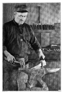
FIG 7-WEDGE IT FAST AND WELD LIGHTLY AT POINT.
