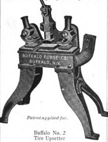
THIS machine upsets 3 x 5% tires and axles up to 1½ in. square. Grips are faced with tool steel with teeth carefully cut and tempered. Lower grips adjust themselves automatically to curvature of tire or for straight work. Upset both straight and curved work. The plunger prevents all buckling or kinking. Weight 275 lbs. Height 22 in. Write for circular.
