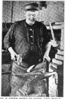
FIG. 8-THEN BEND IT OVER AND WELD.
