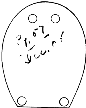
THE FRONT HOOF IS FITTED WITH A PLATE FASTENED WITH CALKS
