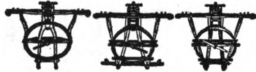
Trussed Platform Wagon Gear Complete, Ready for Body.
