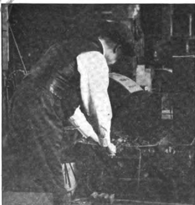
FIG. 3.—INSURE EVEN HEATING BY TURNING THE TOOL IN THE FIRE
