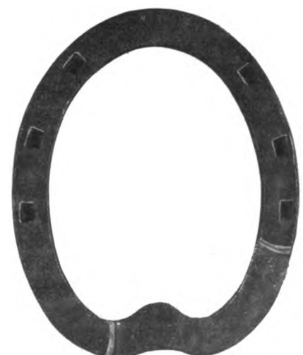
FIG. 2—THE RIGHT BRANCH OF THE SHOE IS THINNED FROM THE GROUND SURFACE SIDE
