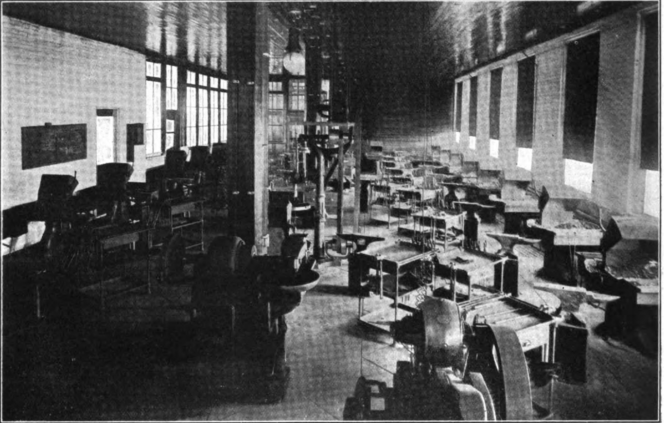
THE FORGE ROOM AT THE UNIVERSITY OF MISSOURI CONTAINS TWENTY-FOUR DOWN-DRAFT FORGES
