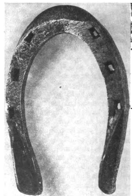
FIG. 3—TAPERED HEEL CALKS ON SHOE TAPERED AT THE TOE
