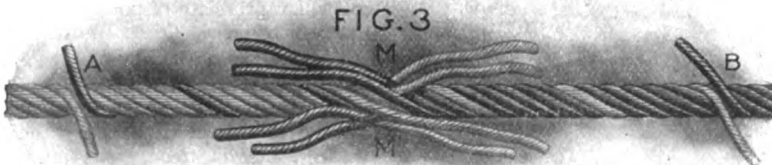
ONE STRAND AT A TIME IS UNLAIDD AND REPLACED BY ONE FROM THE OPPOSITE END
