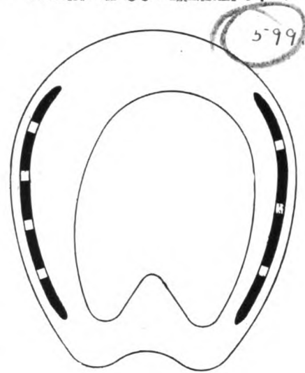
FIG. 4.—A BAR SHOE WITH A SIDE WEIGHT
