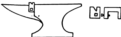
A DIE FOR WELDING SHARP TOE CALKS
