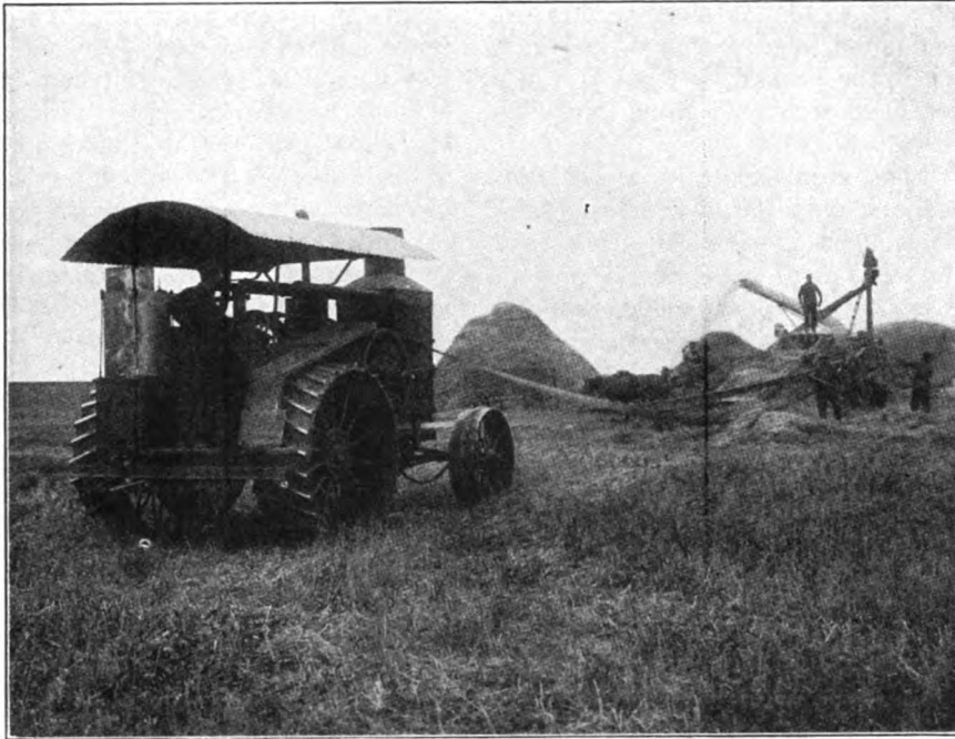
"THE PLOW ENGINE IS ALSO SUCCESSFUL FOR BELT WORK, SUCH AS THRESHING, SHELLING AND SHREDDING"
