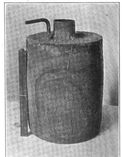
FIG. 3—THE HEATING POT SEALED AND READY FOR THE FURNACE
