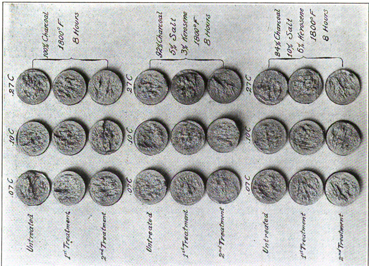
PHOTOGRAPHS WERE TAKEN OF THE FRACTURES OBTAINED FROM THE SAME SPECIMENS THAT WERE USED TO DETERMINE THE DEPTH OF THE FILE-HARD CASE. THESE ENGRAVINGS SHOW THE FRACTURES AFTER FOUR AND EIGHT HOURS OF TREATMENT
