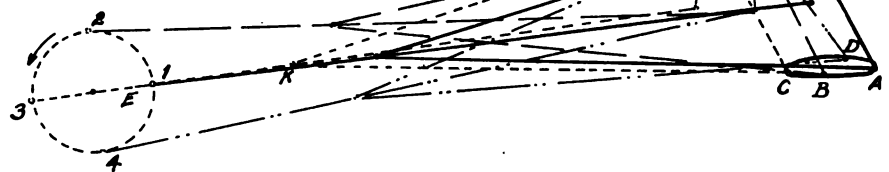
FIG. 1—DIAGRAM SHOWING PRINCIPLE UPON WHICH THE PLOW SHARPENER OPERATES
