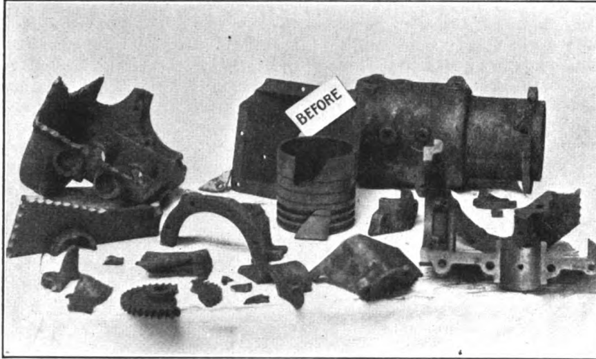
THE BROKEN EDGES ARE GROUND SO AS TO LEAVE A V-GROOVE WHEN PUT TOGETHER. THE PIECES ARE WELDED IN SPOTS TO HOLD THEM IN POSITION. THE LARGE PIECES BEING PREHEATED AND THEN WELDED BY MEANS OF OXY-ACETYLENE
