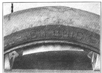
FIG. 7—AFTER APPLYING THE INSIDE FINISHING STRIP, THE TIRE IS PLACED ON MANDREL
