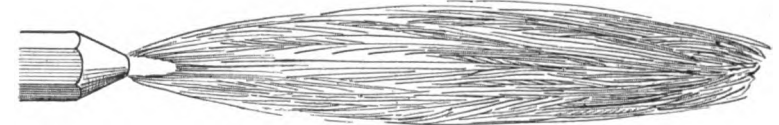
Properly adjusted or neutral welding flame. Cone in centre is sharp and distinct, somewhat blunt. Ragged edges of the rosebud cone of the figure above just disappeared. To test, increase acetylene slightly until rosebud shape begins to appear.
