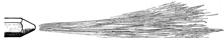
Acetylene turned on with sufficient pressure so that it burns away from the tip slightly—same appearance as "steam" coming from a tea-kettle.
