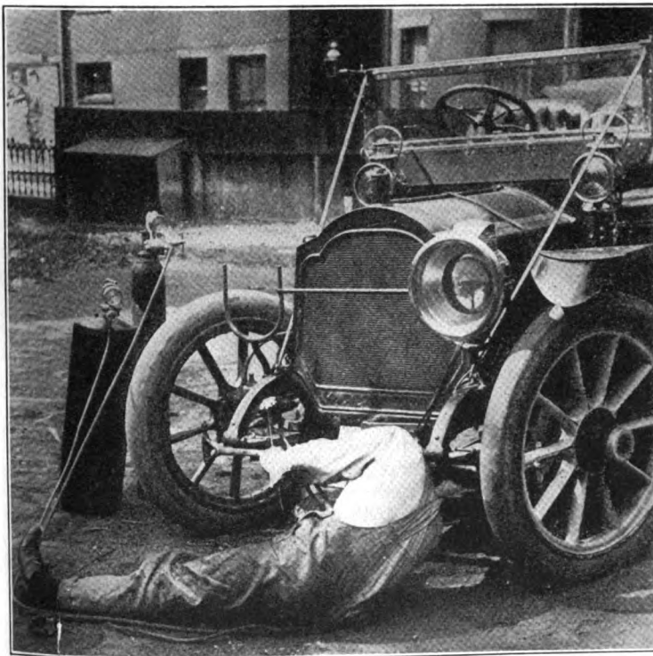
FIG. 7—THE EXTREME PORTABILITY OF THE OXY-ACETYLENE PLANT MAKES FOR REDUCED COST IN PREPARATIONS FOR ACTUAL WORK
