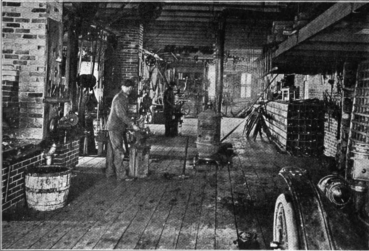
THIS SHOWS THE CARRIAGE SIDE OF THE SHOP WITH THE STORAGE DECK, STOCK RACKS AND BOLT CABINET
