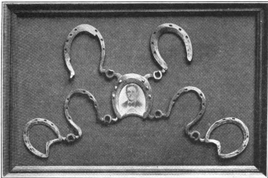
MR. LESTER W. SIMS' HORSESHOE-TURNING STUNT—THIRTEEN SHOES FROM ONE BAR AND WITHOUT A WELD
