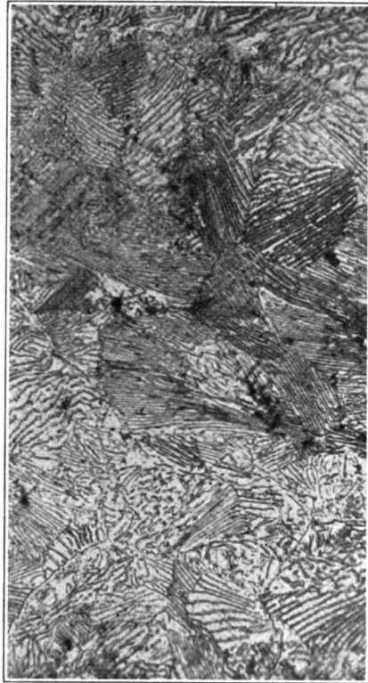
FIG. 2.—THIS STEEL CONTAINS ABOUT 0.85 PER CENT. CARBON; SO THAT IT IS ALL OR NEARLY ALL PEARLITE. THE DARK PORTIONS ARE PURE IRON (FERRITE); THE WHITE PORTIONS, CEMENTITE (IRON CARBIDE). THIS VIEW IS 400 TIMES LONGER AND 400 TIMES WIDER THAN THE STEEL IT REPRESENTS
