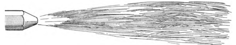
Oxygen turned on, uniting with the acetylene. A cone begins to appear in the centre, shaped somewhat like a rosebud, blue-white in color. This is what is called a carbonizing flame—that is an excess of acetylene or not enough oxygen.
