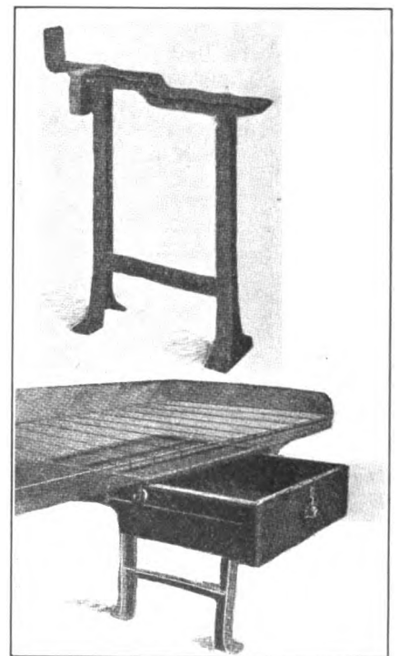
FIG. 4.—CAST IRON BENCH LEG AND HOW USED
