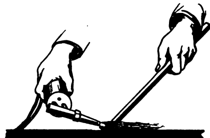
FIG. 17.—HOLD THE TORCH SO THE FLAME JUST STRIKES THE ARTICLE
