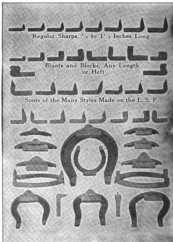
The above is an actual photograph of some of the work, just as it came from the machine without a hammer touching it.
