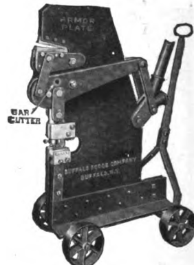
No. 5. Punch, Shear and Bar Cutter Punches ¾ x ½ inch. Cuts Flats, 6 x ¾ inch; Rounds, 1 inch.
