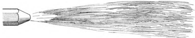
Oxygen turned on, uniting with the acetylene. A cone begins to appear in the center, shaped somewhat like a rosebud, blue-white in color. This is what is called a carbonizing flame—that is an excess of acetylene or not enough oxygen.
