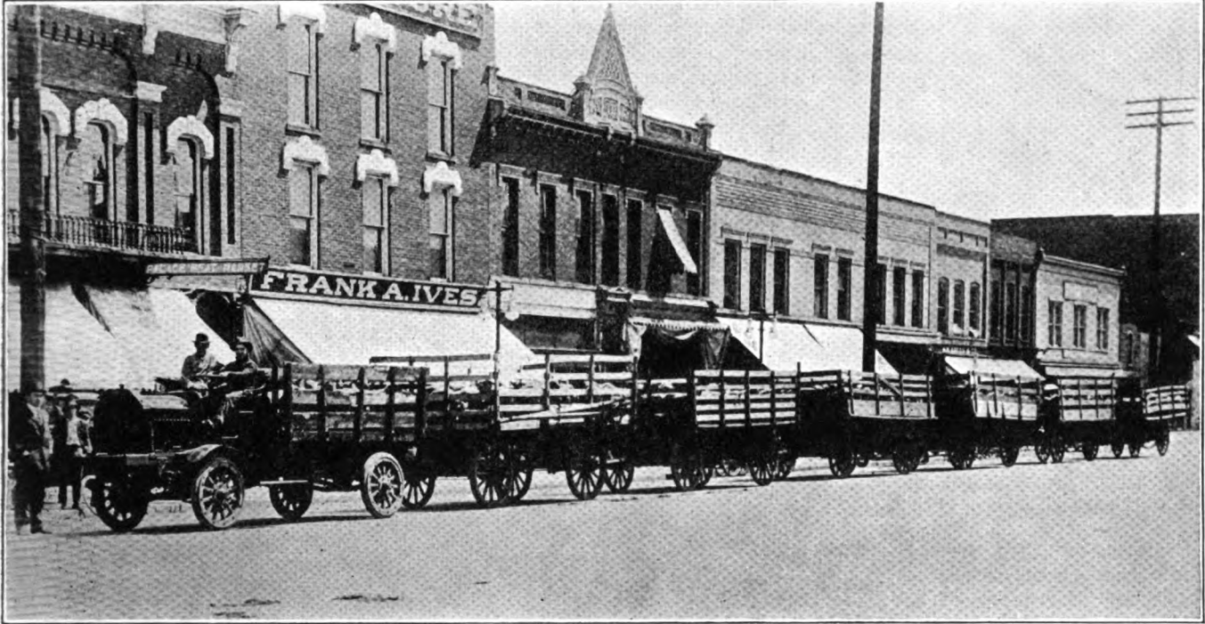
THE MOTOR TRUCK IS REVOLUTIONIZING FARMING AS WELL AS THE INDUSTRIES. HERE WE SEE A TRAIN OF SIX HEAVY WAGONS, HAULED BY ONLY ONE TRUCK, BRINGING 300 SHEEP TO MARKET!
