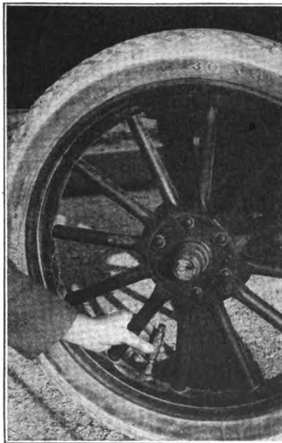
USE A TIRE GAUGE—DON'T GUESS AT THE AIR PRESSURE
