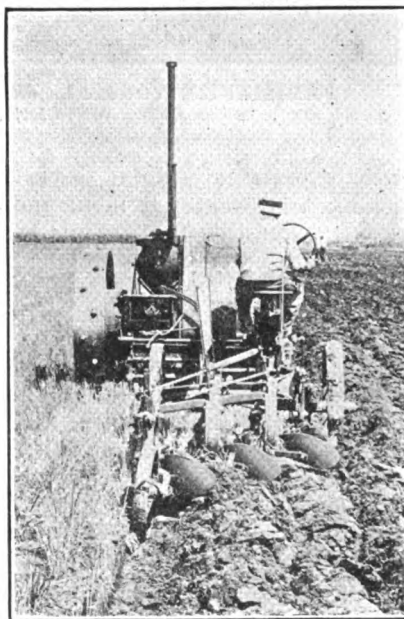
UNDER SOME CONDITIONS IT IS BETTER TO USE THREE PLOWS THAN TWO 14 INCH.
