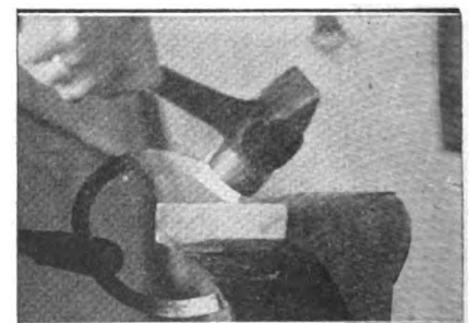
Fig. 12—Bringing heel back to original width after cutting.
