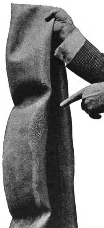
RESULTS LIKE THIS ARE OBTAINED BY USING TOO MUCH POWDER IN THE CASING.
