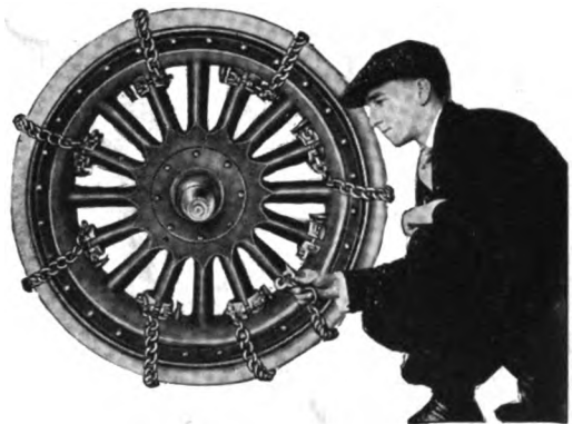
Showing how easy it is, with the patented Prest-O-Grip Lock-Links, to snap Prest-O-Grip chains on and off. As will be seen, the chains lie flat on the tires—due to a special twist in the links. They do not cut the tires.
