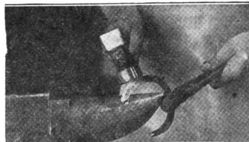
Fig. 19—Shaping the shoe when one heel and a quarter are too narrow.
