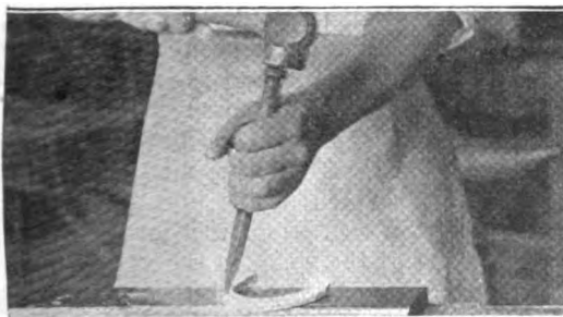
Fig. 16—In punching out nail holes on upper surface, slant pritchel inward.
