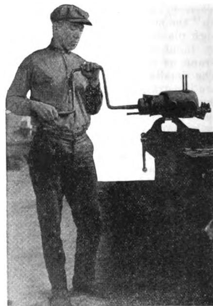
METHOD OF USING THE BRACE AND PISTON FOR LAPPING OUT THE CYLINDERS
