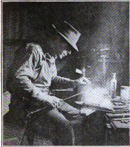
WELDING A DYNAMO OUTER END BEARING AND END SHIELD THAT WAS BROKEN IN THREE PARTS. THE BEARING IS COVERED WITH ASBESTOS TO PREVENT MELTING THE BABBITT
