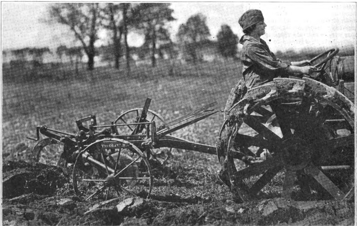
"CLOSE UP" OF THE OLIVER TWO BOTTOM PLOW FOR USE WITH THE FORDSON TRACTOR. THIS OUTFIT IS AUTHORIZED BY THE TRACTOR MANUFACTURER'S AS THE MOST DESIRABLE PLOW EQUIPMENT FOR USE WITH THIS TRACTOR.
