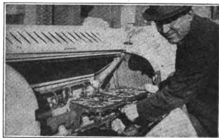
FIG. 5—A GASOLINE STOVE THAT IS ALWAYS IN PLACE AND IS CONNECTED TO THE GASOLINE SUPPLY LINE
