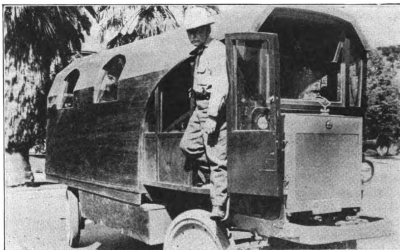
THE COMPLETED BODY WHICH WEIGHS 5,000 POUNDS IS CARRIED ON A FOUR WHEEL DRIVE TRUCK WHICH STEERS, DRIVES AND BRAKES ON ALL FOUR WHEELS
