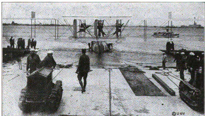
Tractors of the tank tread type hauling the NC-1 from the water just after its last test flight before starting on the first section of its trans-Atlantic flight. Many of the naval air stations have been equipped with the make of tractor shown and which serve a variety of purposes faithfully and well.
