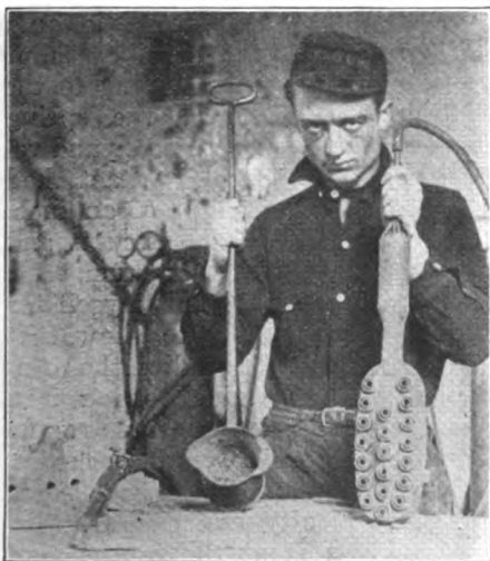
No. 3—THE GAS BURNER AND LADLE, BOTH CONVENIENT ACCESSORIES IN THE WELDING SHOP
