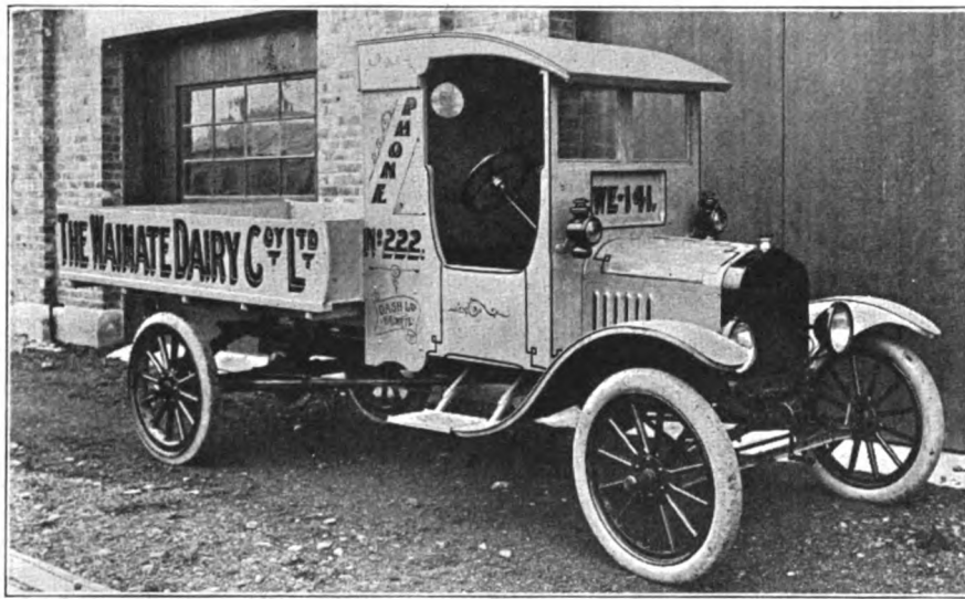
BODY BUILT ON FORD TON TRUCK CHASSIS BY GEORGE DASH—This chassis retails in New Zealand for $1,175 or £235, and the body is built at a cost of $250, or £50. A Ford touring car sells at $1,285, or £257, and a Maxwell for £385, or $1,925.
