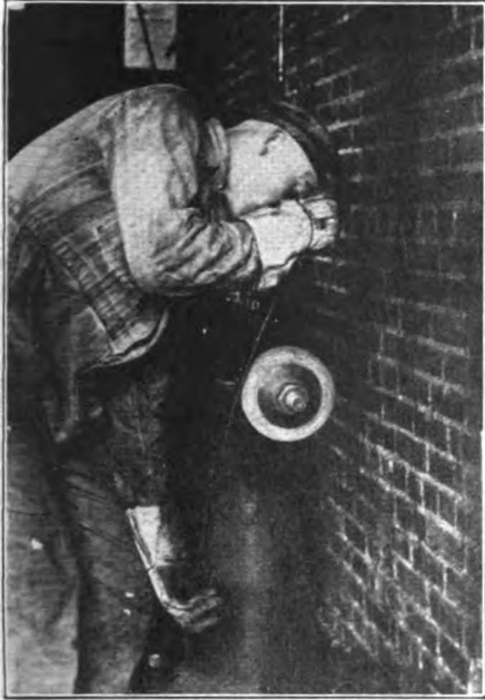
FIG. 3. THE CORRECT WAY TO HOLD THE LEAF FOR GRINDING THE WELD
