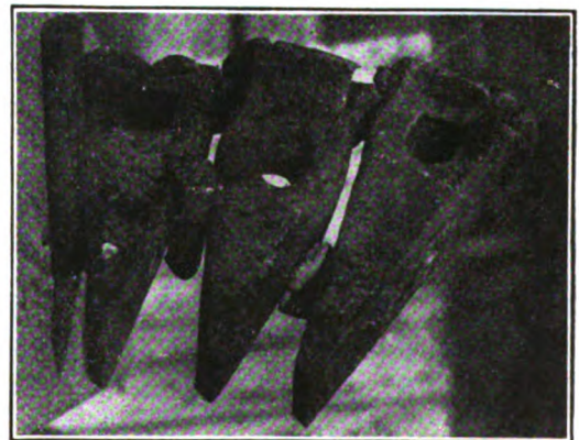
ALTHOUGH THE HEADS ARE BADLY BATTERED THE CUTTING EDGE IS STILL SERVICEABLE
