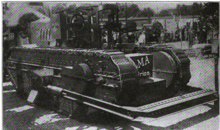
THE GERMANS MAY NOT BE "CONVERTED" BUT THEIR TANKS ARE The illustration shows a corner of a Berlin exposition with a one time tank body rebuilt as an agricultural tractor. The limited size of German farms and the expense of such a machine makes their use very limited. The construction, however, is characteristically and ponderously German.
