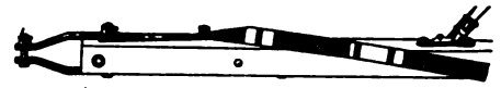
Fig. 5. STUB TONGUE TRACTOR HITCH FOR FIRST BINDER OF TWO, SHOWING CLEVIS AND STUB TONGUE
