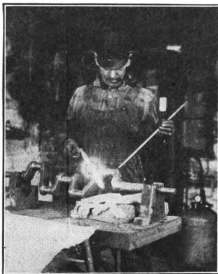
THE GENERAL ARRANGEMENT OF V BLOCKS AND ASBESTOS REFLECTOR USED IN WELDING A BROKEN CRANK SHAFT
