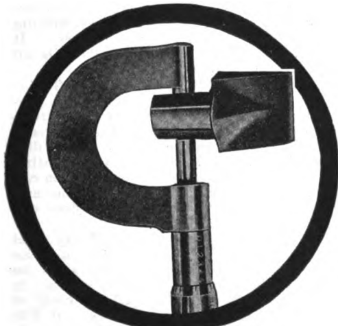
The shanks and calk holes are so accurate as not to vary 1-10,000 of an inch in diameter.
