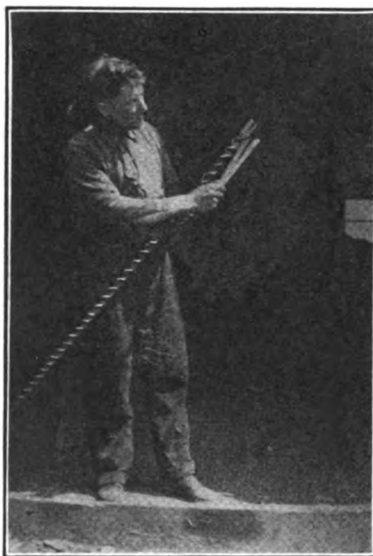
Fig. 2. THE FIRST STEP IN SHARPENING THE COAL AUGER
