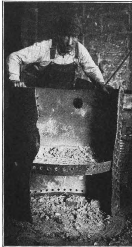
HOME-MADE PREHEATER. VERY HANDY FOR COKE DESPITE ITS CRUDE APPEARANCE
