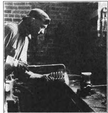
FIG. 2—METHOD OF MAKING RODS OUT OF COIL SPRINGS
