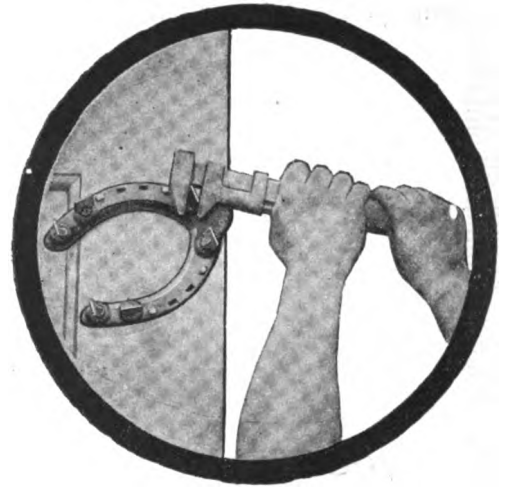
The same man's entire weight failed to twist this calk so much as a hair.
