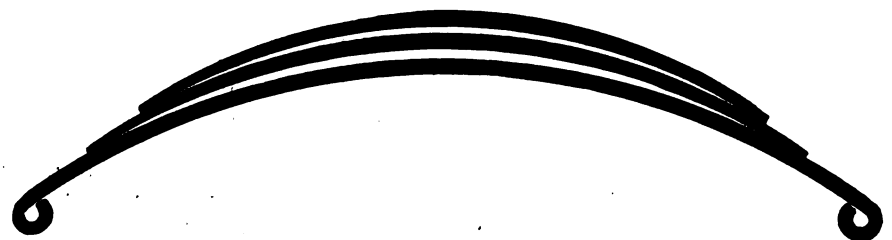
FIG. 5 SHOWING THE PROPER SPACING BETWEEN THE MAIN AND SECOND LEAVES. THE SPACE BETWEEN THE MAIN AND SECOND LEAF IS THE THICKNESS OF ONE LEAF. THE SPACE BETWEEN THE SECOND AND THIRD LEAF IS SLIGHTLY REDUCED AND SO ON UNTIL THE LAST TWO FIT FAIRLY SNUG.
