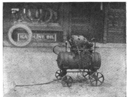
MOUNTED ON ITS OWN TANK AND ELECTRICALLY OPERATED THIS OUTFIT CAN BE TAKEN ANYWHERE
