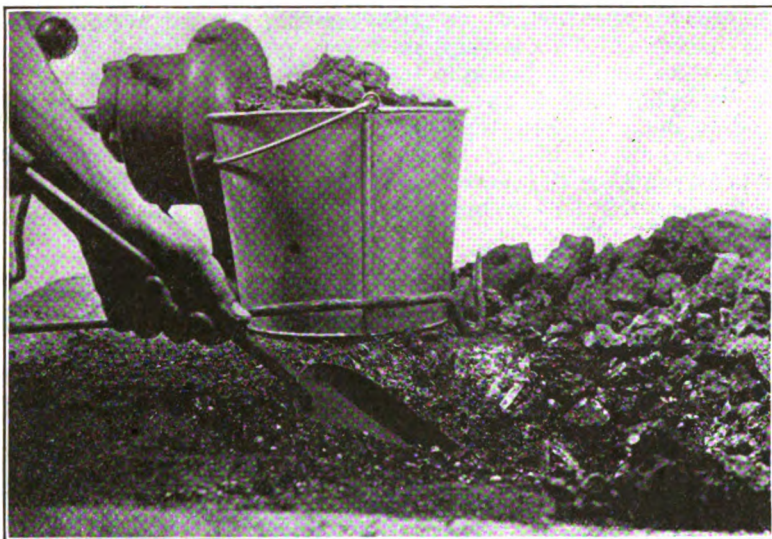
FIG. 2.—THE COKED COAL FROM THE OLD FIRE SHOULD ALWAYS BE SAVED AS IT MAKES A HOTTER AND BETTER FIRE FOR WELDING
