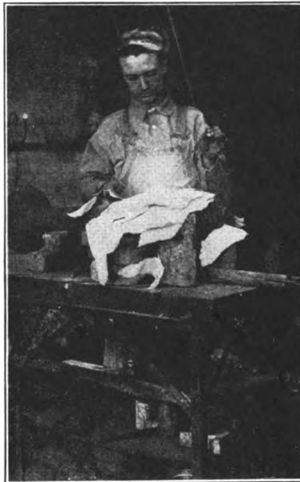
FIGURE 2 SHOWS HOW THE PART WAS COVERED WITH ASBESTOS TO RETAIN THE HEAT
