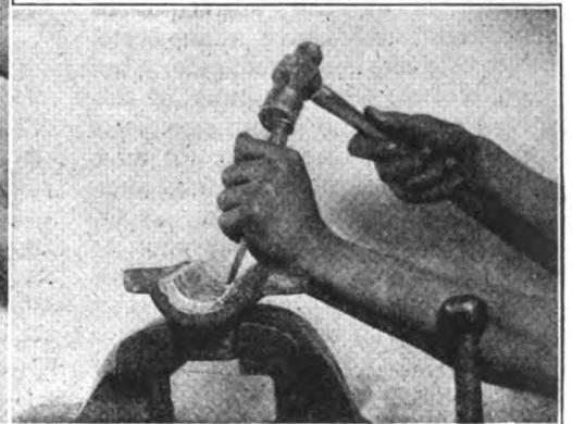
FIG. 15—LAST OPERATION IS THE CUTTING OF OIL GROOVES
