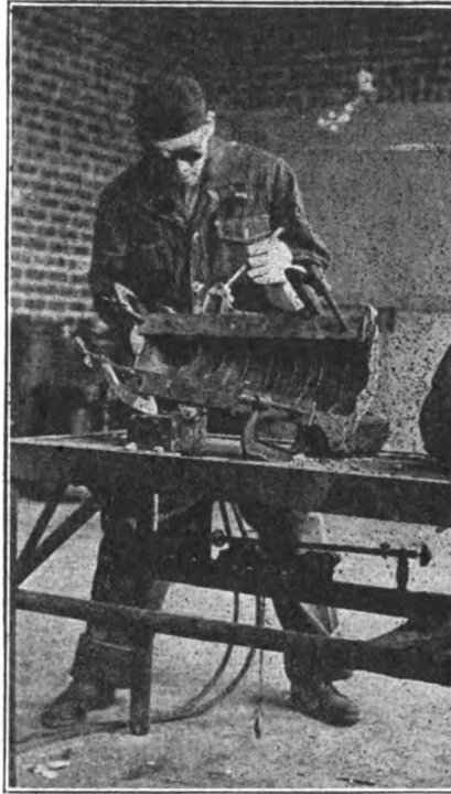
FIG. 2.—CLAMPS ASSIST IN HOLDING THE CASE WHILE WELDING
