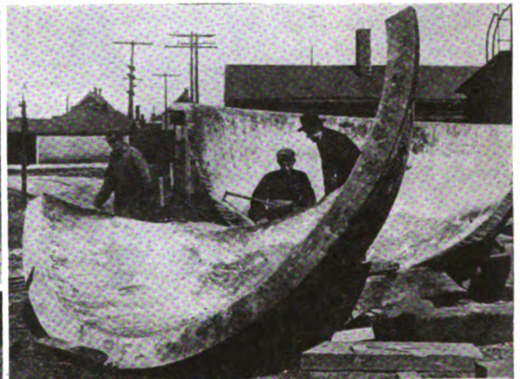
TOP LEFT — CUTTING CAST IRON WITH THE CUTTING BLOWPIPE. TOP RIGHT — SIXTEEN TON CAST IRON MELTING POT CUT IN TWO IN TWO HOURS AND THIRTY-FIVE MINUTES. THE POT WAS TWELVE FEET IN DIAMET-
