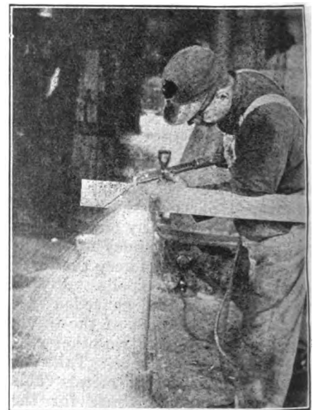
Fig. 3. CUTTING HEAVY ANGLE IRON FREE-HANDED. NOTE THE REGULARITY OF THE FIRST CUT
