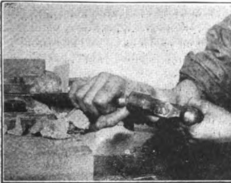
FIG. 11—THE CAP IS REMOVED AFTER BEARING IS COOL
