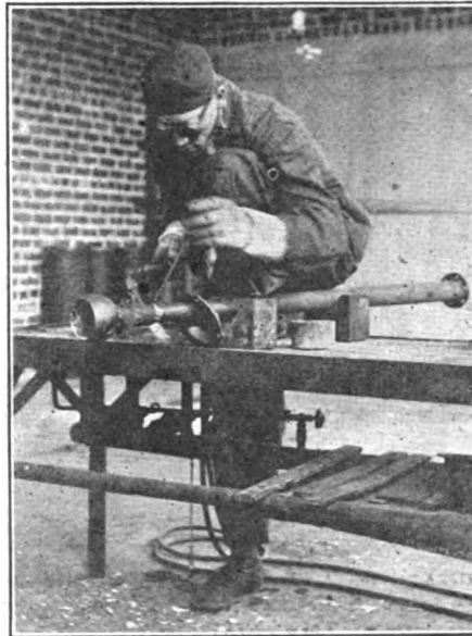
THE MALLEABLE PART OF A DRIVE SHAFT HOUSING BEING BRAZED IN PLACE.
