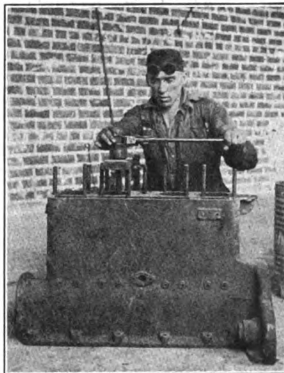
FIG. 1—THIS IS HOW THE SLEEVES WERE PULLED OUT OF THE BLOCK
