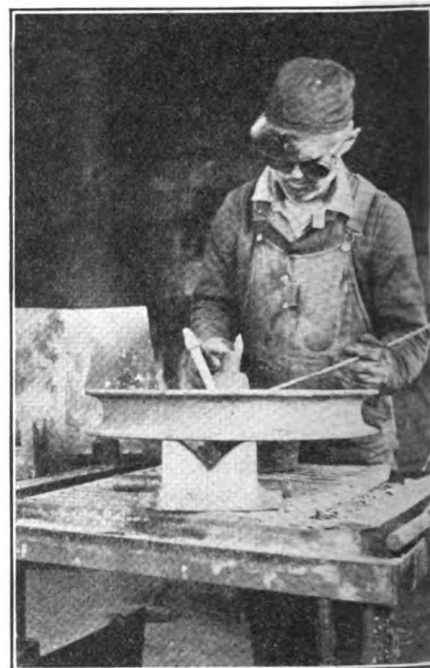
FIG. 3. THE FIRST WELDING POSITION OF THE BROKEN WHEEL
