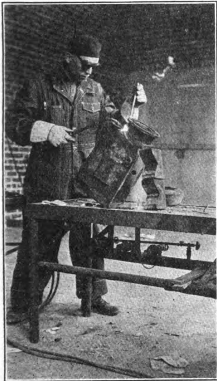
FIG. 2.—THE NECK WAS WELDED WITH THE PREHEATING FLAME INSIDE THE CASE.
