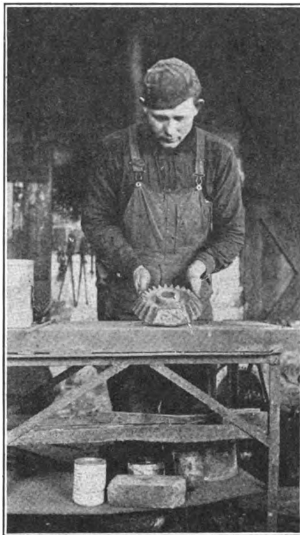
FIG. 3. THE BROKEN TEETH WELDED "EN BLOC".
