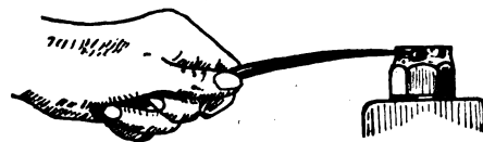
COTTER PIN EXTRACTOR MADE FROM OLD FORK TINE.
