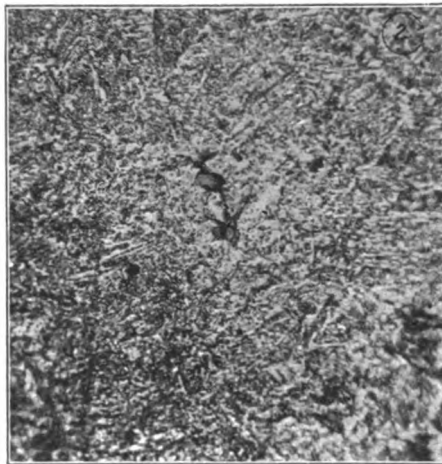
Fig. 2. Strained piece of gun steel showing rupture beginning at small defects, two small dots of manganese sulphide.
