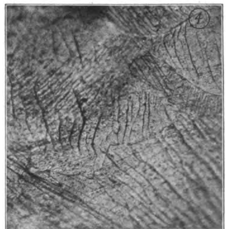
Fig. 4. Armco iron strained. The curved lines are not cracks, but the edges of parts of the grains that have slipped past each other, so that the surface of each grain is stepped, as would be the top of a row of books that had slid past each other. In some grains there are two sets. They are called slip bands.
