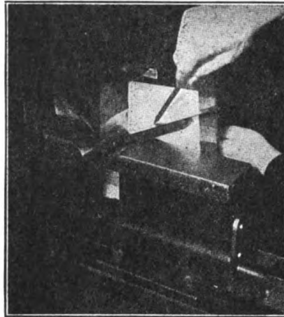
FIG. 14—MEASURING THE ANGLE IN BENDING TEST
