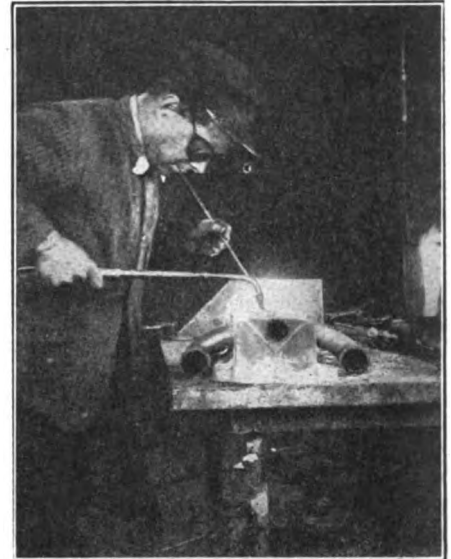
Fig. 3. FILLING THE GROOVE
