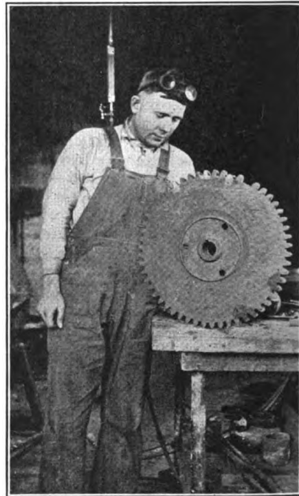
Fig. 2. THE REPAIRED TEETH IN DIFFERENT STAGES OF THE OPERATION
