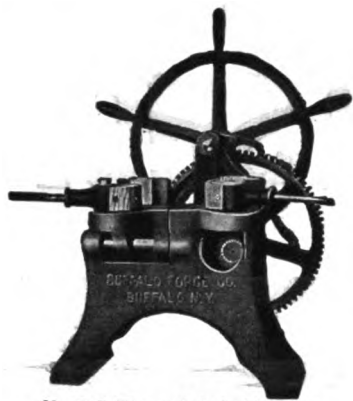
No. 3-G Tire and Axle Upsetter
