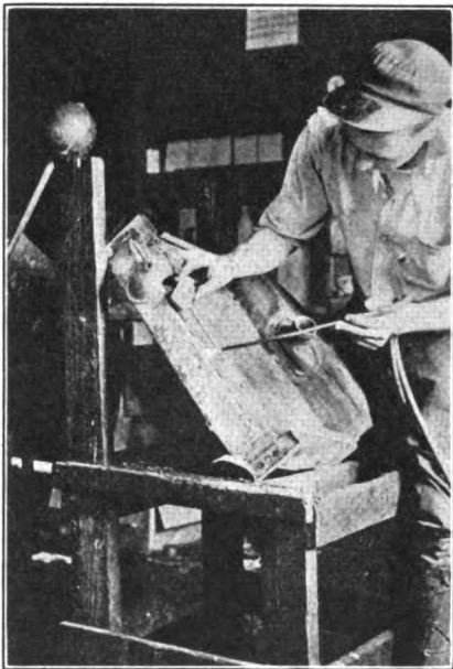
FIG. 4—USING THE LEAD-BURNING TORCH TO REPAIR RADIATOR LEAKS
