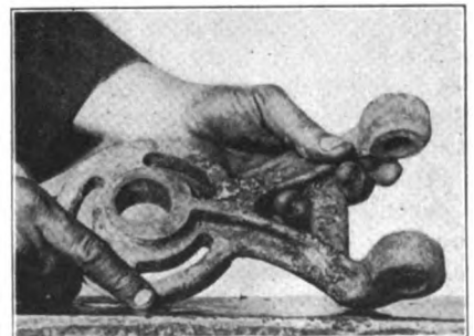
FIG. 11—AFTER COOLING THE CASTING IS CLEANED UP WITH A FILE
