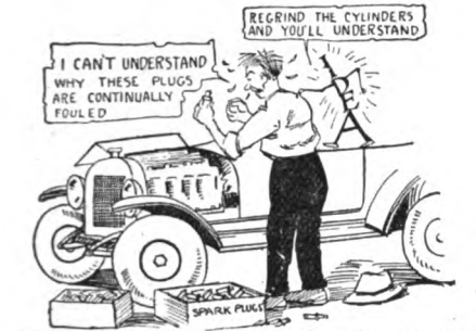
CARBON FORMATION IN THE CYLINDERS WILL BE CORRECTED BY REGRINDING
