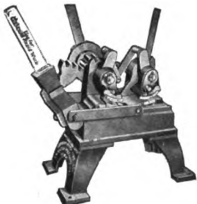
The C-O No. 1 1/2 Tire and Axle Shrinker takes from the smallest up to 4"x1" round edge tires and 1 1/4" square axles. Special gearing applies full load with a minimum of effort.
