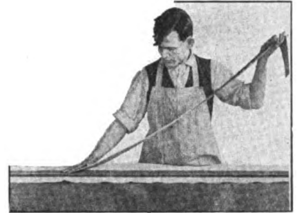
FIG. 27—THE NEW TREAD IS BUILT UP FLAT ON A TABLE BEFORE APPLYING
