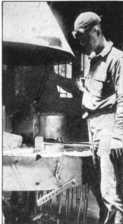
FIG. 2—THE CYLINDER WAS PLACED IN THE FORGE FIRE FOR PREHEATING
