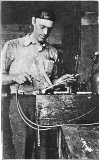
FIG. 2—ANOTHER USE FOR THE LEAD-BURNING TORCH IS IN ATTACHING NEW BATTERY CONNECTORS
