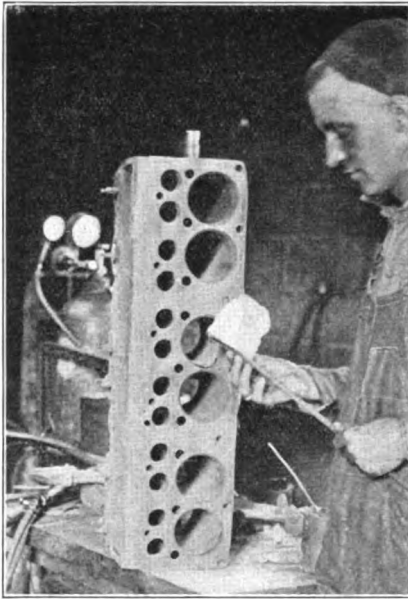
FIG. 2—CLEANING THE SCORES WITH SAND PAPER WRAPPED AROUND THE SCRAPER
