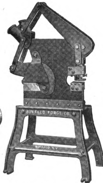
3B Punch and Shear Punches \frac{3}{8} \times \frac{3}{8} Cuts \frac{3}{4} rounds or 3 \times \frac{1}{2} in. flats.
