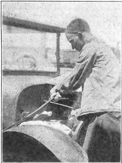
AN ASBESTOS PAD HELD BY MEANS OF A ROD OR WIRE WILL DEFLECT THE SPARKS
